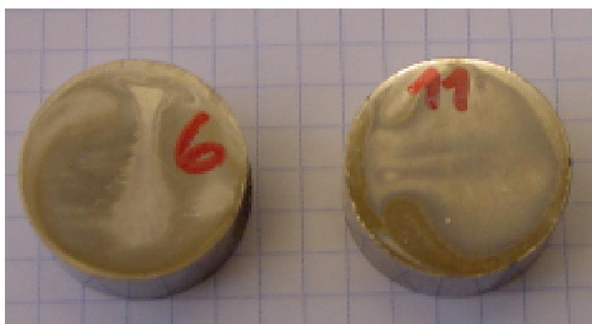
*Fig. 5.2:* Flame-like surface defects on electroless nickel-boron deposits synthesized in the early deposition cell.
