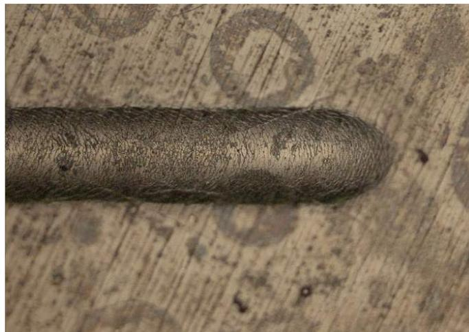
Fig. 8.30: Residual scratch on electroless nickel-boron coated aluminum (maximal load: 25N) - end of the scratch.
