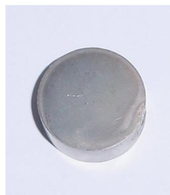
Fig. 2.2: brightness of an electroless nickel-boron deposit.
