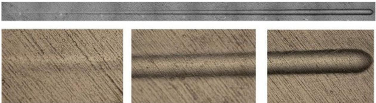
Fig. 9.21: Scratch test on a electroless nickel-boron coating after heat treatment at 180°C.
