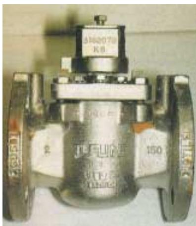
*Fig. 4.1:* Electroless nickel coated control valve.[117]
