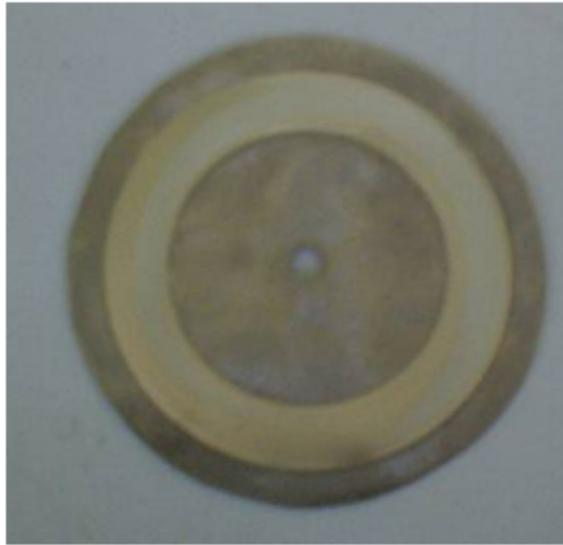
Fig. 8.23: Aspect of a sample after Taber testing.
